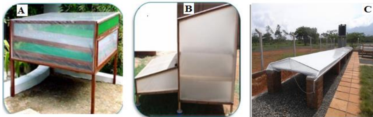
Plate 1. Different solar dryers used in the study: (A) Cabinet direct dryer-CDD, (B) Cabinet mixed mode dryer-CMD and (C) Hoenheim Tunnel dryer-TD.
